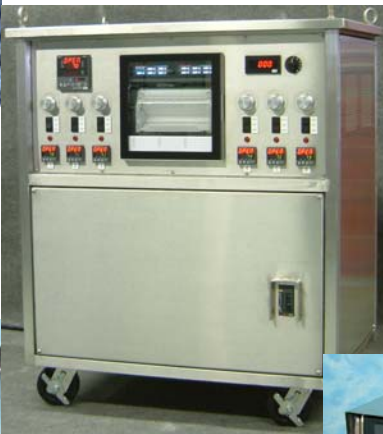
6 Way Heat Treatment Console
