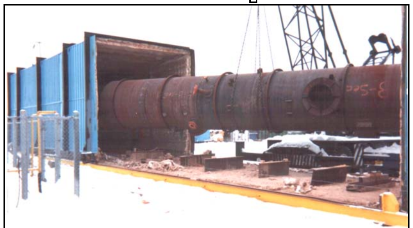
50' L x 15' W x 16H High Velocity Gas Furnace located at 30 Estates Road.
