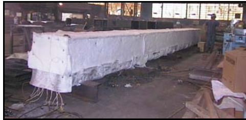
30' Box beam wrapped and electrically pre-heated at customer's facility.
